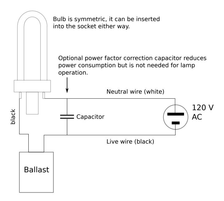
Ballast is symmetric, it can be wired either way, both wires are equivalent.
